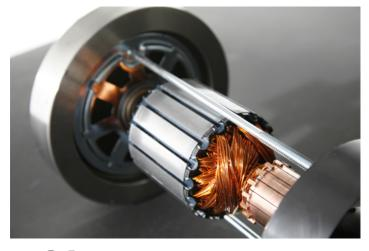
**O1** 2.0 CHP DurX<sup>™</sup> MOTOR The 2.0 CHP Motor features dual fans that cool internal components while running for less noise and vibration, while superb insulation and a built-in grounding brush ensure the motor performs with quiet reliability mile after mile.
